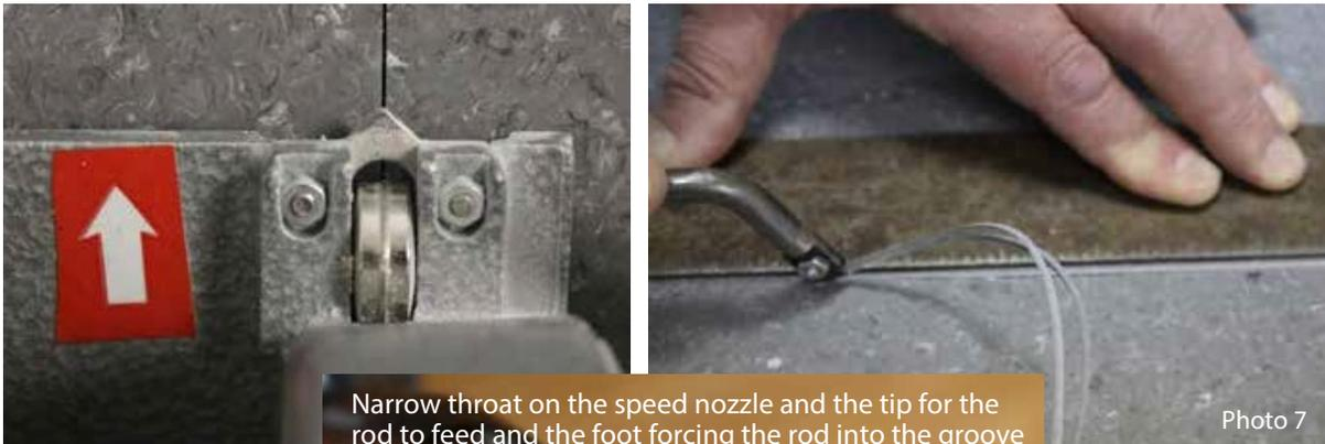
through the nozzle's tip during the welding process. Please notice in **Photo 8** (on previous page) that the throat of the speed nozzle is narrow. The purpose of the nozzle is to uniformly heat both the welding rod and the groove to a pre-determined temperature so that the physical "melting of the rod to the flooring" is uniform, consistent, without damage and without interruption.
